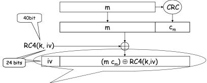
ciphertext: transmitted through the radio link
