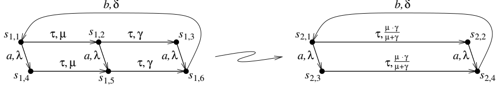
Figure 7: GW-lumpability is not exact in this case due to a non-joining synchronization
